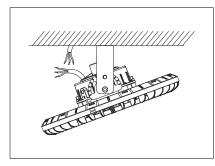
4.Adjust the proper angle of lamp, tighten the nut and connect according to the corresponding wire.
