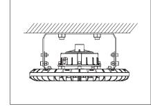
3.Install the lamp bracket on the prearranged wall screws and tighten the nuts.
