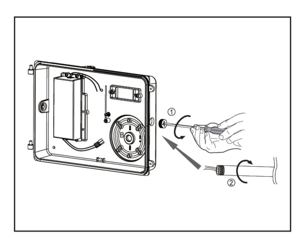
1. Loosen screws and remove the front lens set carefully from the back plate. (See step 1 above)
