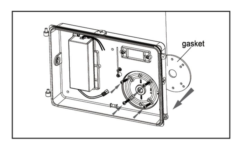
3. Attach the back plate on the wall, use the supplied gaskets for a weather tight seal.
