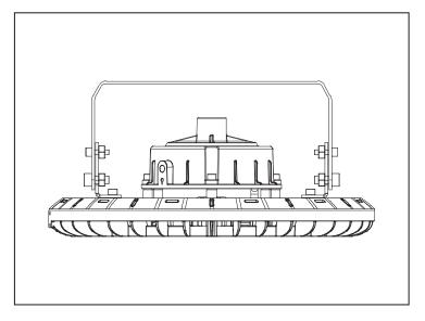
2. Screw the U-shaped bracket onto the bracket fixing plate.
