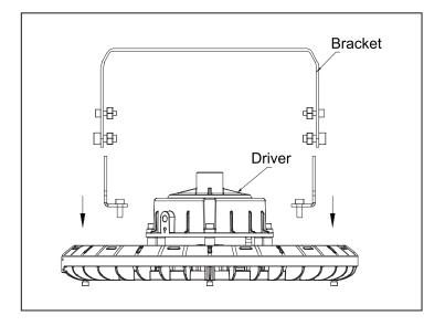
1.The bracket fixing plate is screwed to the lamp.
