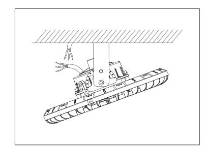
4. Adjust the proper angle of lamp, tighten the nut and connect according to the corresponding wire.
