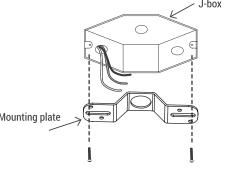
3 Completing the installation by attaching the fixture into the mounting plate tightly to the j-box. Attach the diffuser by twisting and lock the diffuser in place.
