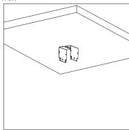
1. Fix the mounting bracket to the ceiling with screws.
