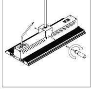
1. Place the mounting bracket to the light fixture, and tighten with a screwdriver.
