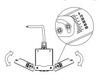
Adjust to angle (0-60°) and secure with a screwdriver.
