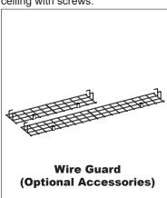
1. Slide the Wire Guards into the two sides of lighting fixture, fasten with screws.
