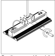
2. Pass the power cord through the one end cap of the mounting bracket, and fix it with screws.
