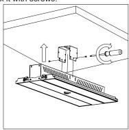
2. Secure the lighting fixture to the mounting bracket, fasten with screws.
