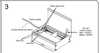
Install the included strain relief bushing in the appropriate hole then push the wires through the connector. Make connections in the compartment: match the white wire from the line feed with the white wire from the LED driver, match the black wire from the line feed with the black wire from the LED driver with the included wire connectors, match the copper wire from the line feed with the green wire from the LED driver
