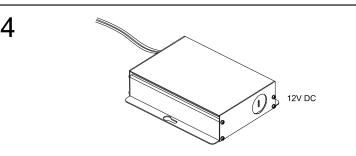
Close the cover, then connect the fixture to the output wire where red wire is (12VDC+) & black wire is 12VDC-
